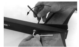
Install a bolt set (the ones saved from disassembly) in the forward holes. Do not tighten yet.
