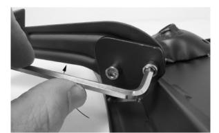
Attach right side support to right-side platform bracket as shown. Tighten securely.
