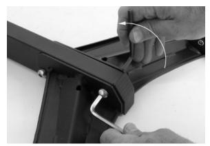
Install a bolt set to the rear holes. Using the supplied hex key wrenches, tighten BOTH forward and rear bolt sets securely.
